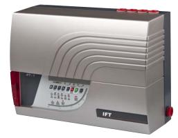
The ICAM IFT-1 detector is an air-sampling system with an alarm sensitivity range from 0.001% to 20% obscuration/m (0.0003% to 6.10% obscuration/ft). This detector is classified as a Very Early Warning Smoke Detector and can reliably detect fire at an early stage, and low to high concentrations of smoke over an area of 2000 m<sup>2</sup> (21 500 ft<sup>2</sup>).
